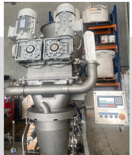
Unique dust extraction system to connect with customers filter system
