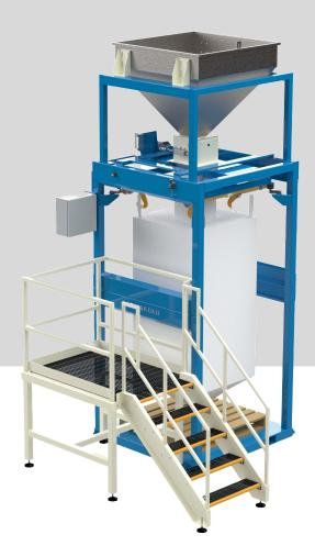
This system is designed for the operator to hang the bags from one side. This system facilitates easy bag handling for operators. The hanging hooks conveniently move towards the operator side, allowing them to easily hook the bag loops on. Then retract, ensuring that the bag hangs freely and the bottom corners fill evenly with product.
