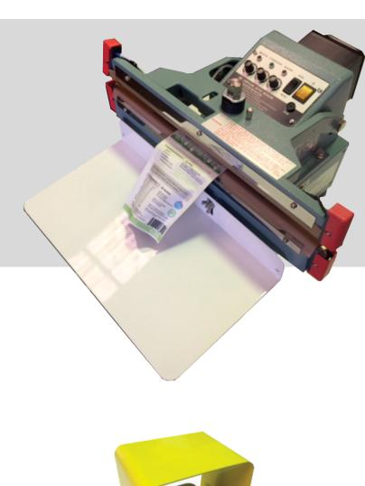
The Innoseal P-450 is a pulse sealer, meaning the element is only energised while the seal jaws are closed. To operate you simply press a switch to close the jaws & engage the sealing it will release automatically.
