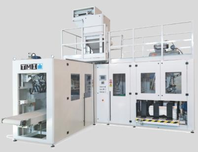
The ILERSAC W is designed to handle bags at high speed with maximum reliability by avoiding lineal transitions at vacuum systems. All handling process is done through pincers that take the bag for all handling process providing maximum control.
