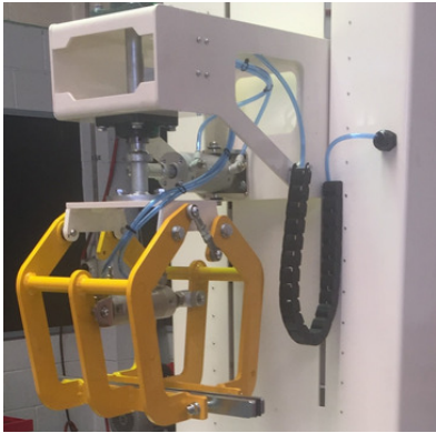
Innotran IT Inline bag turner that grips the bag by the top & turns the bag.
