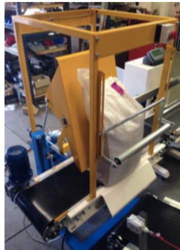
Innotran B 90 degree bag transfer from bagging conveyor exiting with the bag bottom first.
