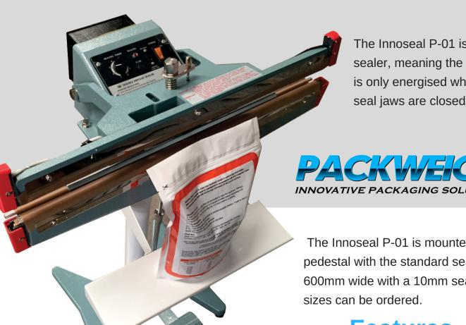
The Innoseal P-01 is a pulse sealer, meaning the element is only energised while the seal jaws are closed.
