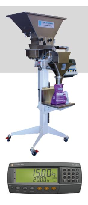
The Innofil VPN is a vibratory feed bagging scale for granular products needing higher accurate weights. This machine is particularly suited to small bags & buckets.
