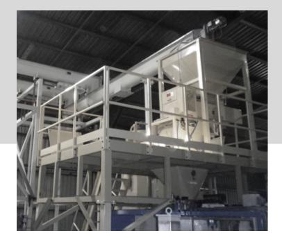
The Innofil B-31 is designed for bagging products with irregular shapes that don't flow well, when high accuracy is needed.
