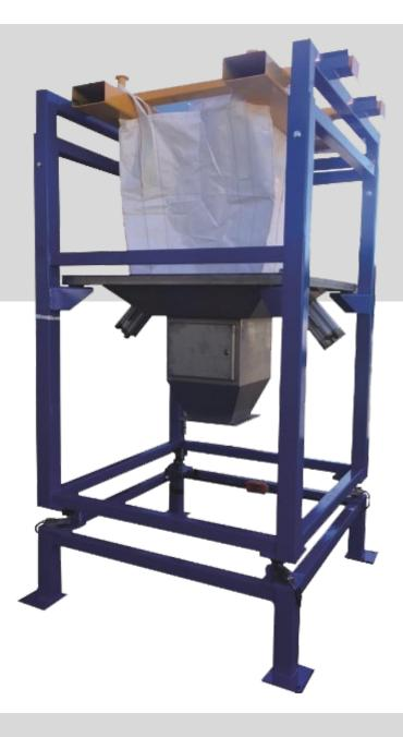
Packweigh manufacture bulk bag unloading systems with or without load cells & weigh controls if you need to remove a certain amount of product.
